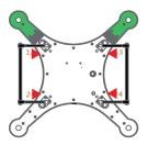
Insert the landing gear one leg at a time, according to the red arrows. Ensure the legs are fully inserted.
