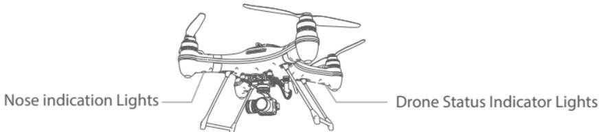
The nose LED indicator lights are always lit and are used to indicate the direction of the nose of the drone. The rear aircraft status lights indicate the current status of the flight control system by flashing patterns of red, green and yellow lights.
