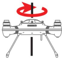
Compass Calibration must be completed within 90 seconds and while the Drone Status Indicators are fast-flashing Red-Green-Yellow.
