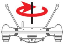
5. Turn the drone **upside-down**, then rotate the drone around you in a **clockwise direction** one full rotation (360 degrees).
