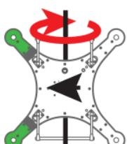
9. Turn the drone **nose left (9 o'clock)**, then rotate the drone around you in a **clockwise direction** one full rotation (360 degrees).
