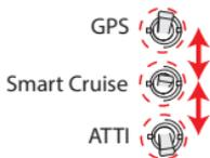
**Two-Sided Compass Calibration Switch Command**
