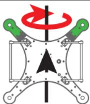
6. Turn the drone **nose up**, then rotate the drone around you in a **clockwise direction** one full rotation (360 degrees).
