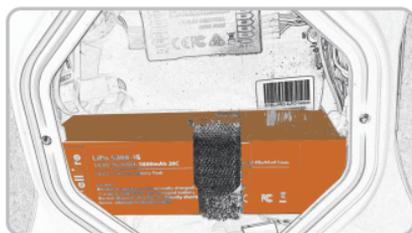
⚠ Once connected to the drone, the battery cables and connectors must be placed in the space between the battery and the rear case of the drone.
