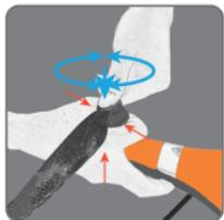
⚠ When installing or removing the propellers, place one hand under the motor to support it when installing or removing propellers.
