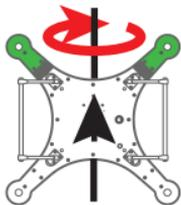
6. Turn the drone **nose up**, then rotate the drone around you in a **clockwise direction** one full rotation (360 degrees).
