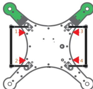
Insert the landing gear one leg at a time, according to the red arrows. Ensure the legs are fully inserted.
