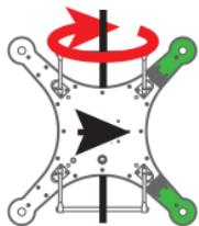
7. Turn the drone **nose right (3 o'clock)**, then rotate the drone around you in a **clockwise direction** one full rotation (360 degrees).
